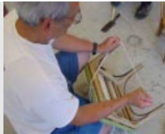
Check the symmetry with a string..
